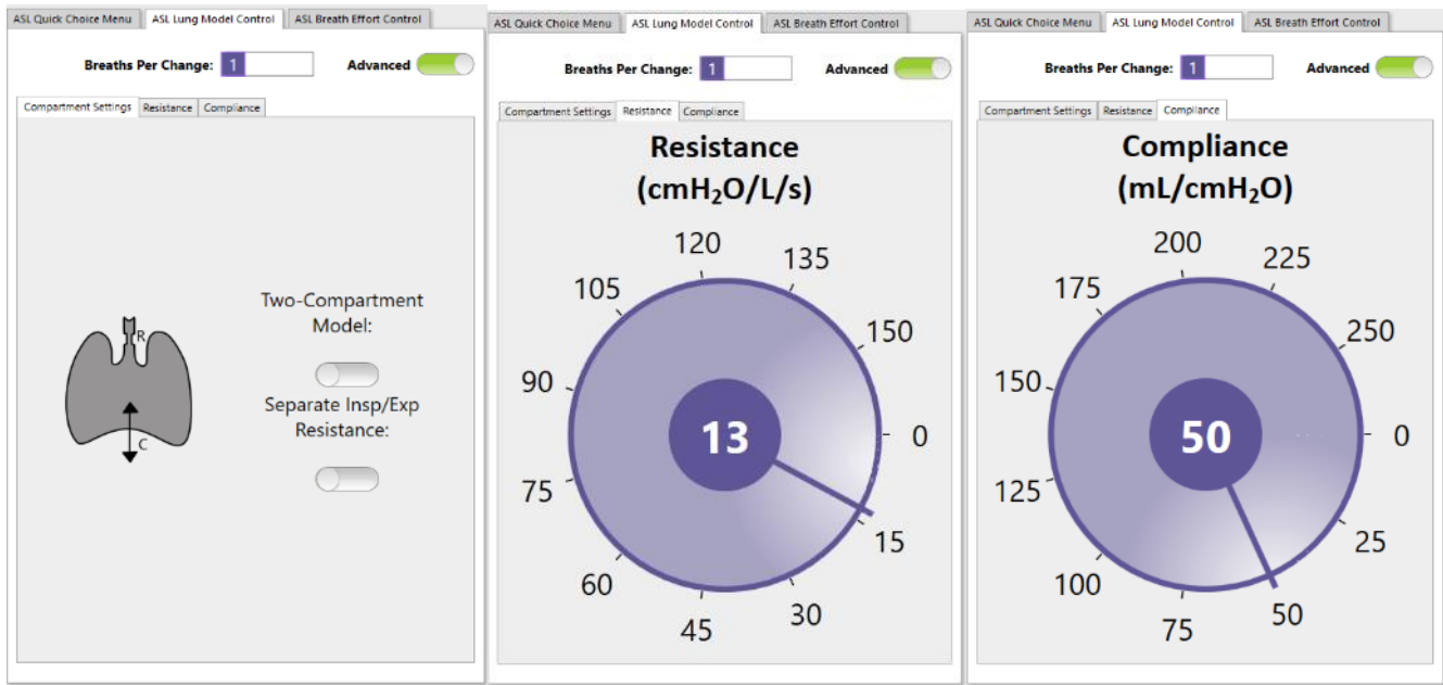
Figure 5-33 - Lung Model – Simplified Lung Model 1 Compartment with Equal Resistances
